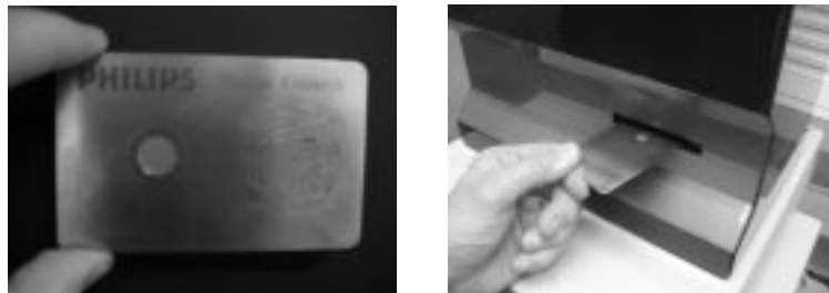
Fig. 1. Left: Card equipped with an optical PUF. Right: Reading device.
